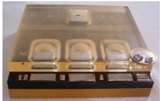
Figure 4 A scale model of a cell counting structure made using a microBUILDER service. The designer participated at a microBUILDER course before designing the device. The device has later been adopted as a design example by the project. On top of the scale model is a 1 Euro coin with two devices on.
