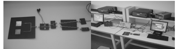
Figure 6 All Rx Blocks of the network (left side) and final test with the two PC's (right side)
